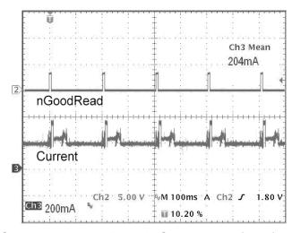
Figure 30. Continuous Image Decode Current Waveform (I\_ave = 204mA)
